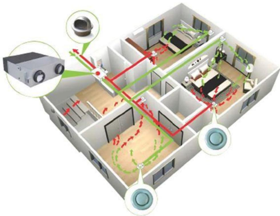
When planning where the pipes/ducting should go remember that it is optimal for the room vents to be situated as far away from the door to the room they are in as possible. Also, in all cases make sure there is an adequate gap between the exhaust vents and the incoming vents to maximise effectiveness.
